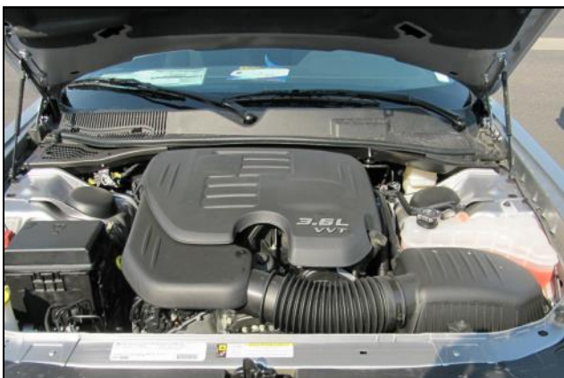
7. Reinstall the intake tube and engine cover in the reverse order that they were removed. Make sure to reconnect the temperature sensor.
